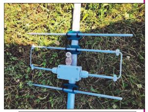
Close up of the driven element of one of the Loop Fed Yagis
